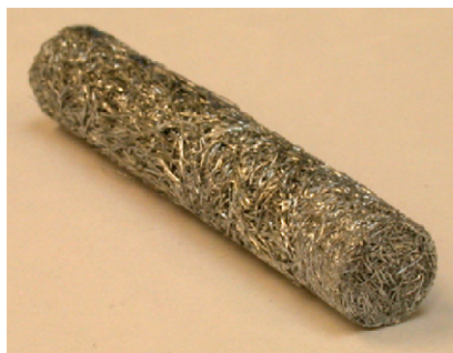
Fig. 3. A rod form of fibrous electrode for an AA cell and a plate form of anode for a large mechanically rechargeable zinc–air cell.
